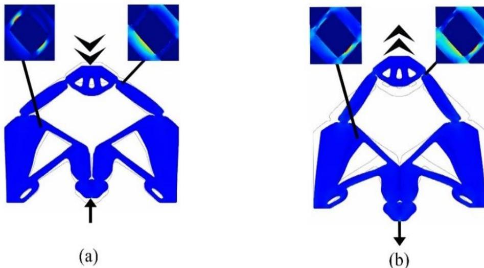
**Figure 5:** Concurrent multiscale design of displacement inverter (a) under compression (b) under tension
