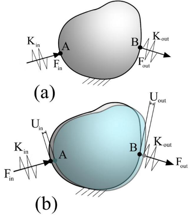
**Figure 2:** Compliant mechanism design problem
