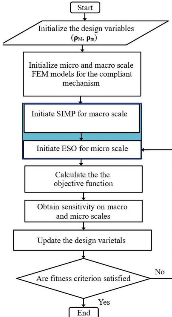
**Figure 3:** Flowchart of concurrent multiscale displacement inverter optimization
