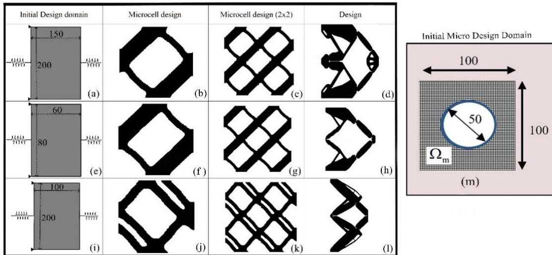
**Figure 4:** Designs domain and the macro and microscale designs
